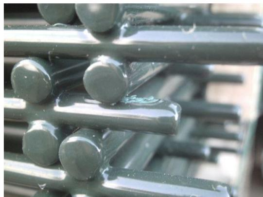
Paint damage by shifting
